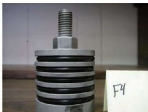
Figure 3 F4 Material installed on Tooling After Test
